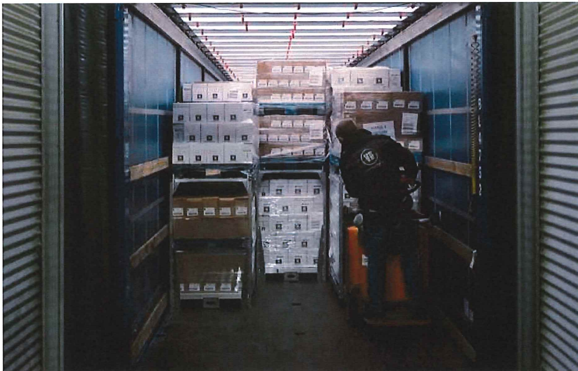
Tests have been done at Midsona's facility in Mariager, Denmark to double-stack pallets to thereby better use the transport space.
